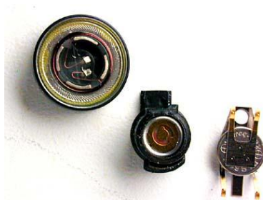
The cell-phone speaker, microphone and battery backup
